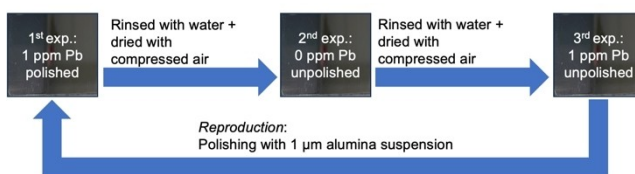
Figure 6. Experimental procedure to investigate if Pb deposits irreversibly onto the electrode during electrolysis and thus activates it.
